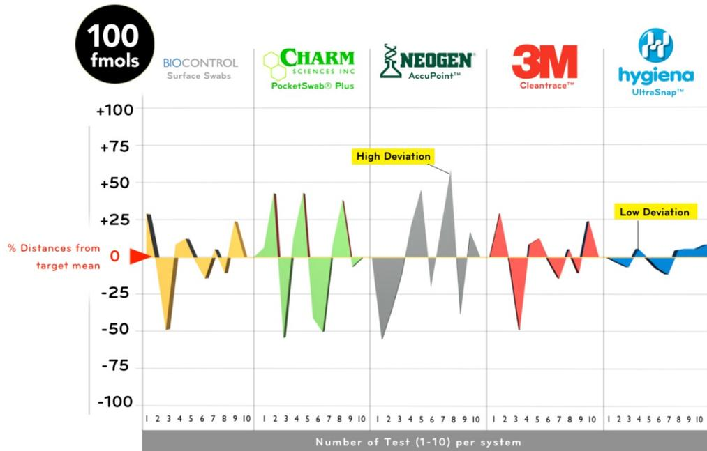
Recommended Pass / Fail limits are usually set close to 100 fmols ATP so good repeatability is essential at this critical value.
