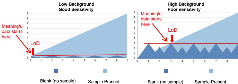
Background noise is interference from the instrument and swab device that gives a positive RLU reading when there is no ATP present - sometimes referred to as false positives. High background noise is commonly seen with photomultiplier tubes
